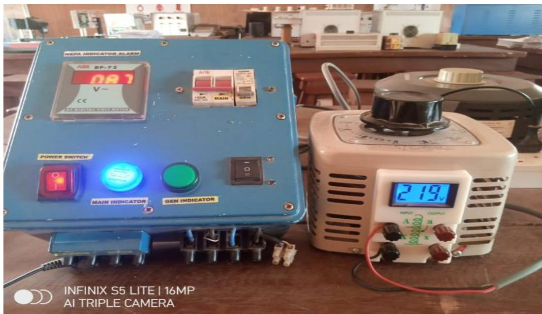
Figure 6: Testing of the system with variarc
